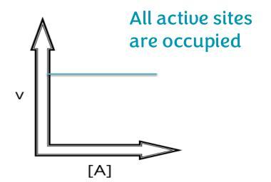
Velocity independent: In a zero-order reaction, the rate is constant and does not change with [A].
