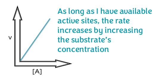
Velocity dependent: In a firstorder reaction, the rate increases as [A] increases.
