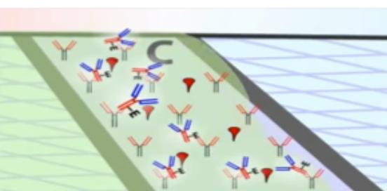
6. The C-zone immobilize them and the enzyme linked antibodies catalyse on with the dye this zone is important to check if the strip is working
