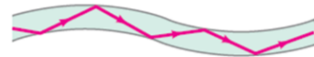
FIGURE 23-29 Light reflected totally at the interior surface of a glass or transparent plastic fiber.
