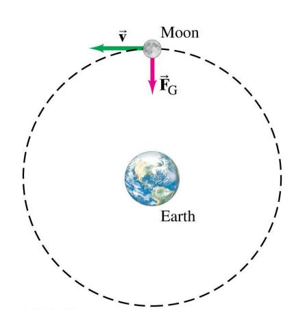
Centripetal forces do no work, as they are always perpendicular to the direction of motion.
