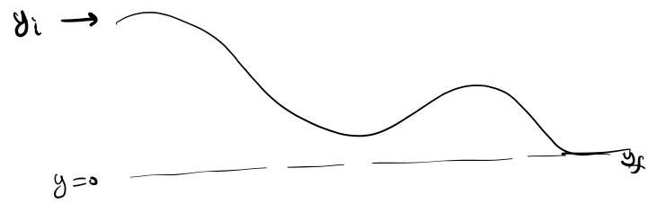
conservative force > work done does not depend on the actual path travelled by the particle, it depends only on the mitial and final points. <u>ex</u>: gravitional force Nonconservative force: the work done depends on the actual path ex: friction force
