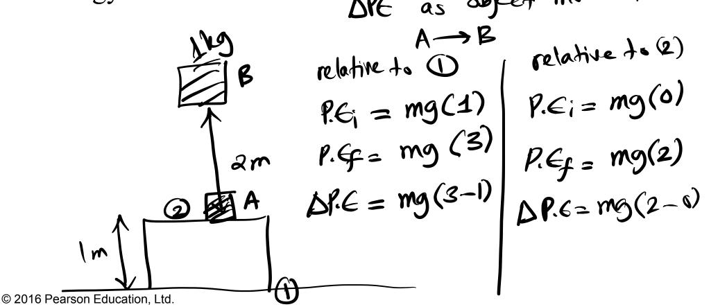
A 1.60-m-tall person lifts a 1.65-kg book off the ground so it is 2.20 m above the ground. What is the potential energy of the book relative to (a) the ground, and (b) the top of the person's head? (c) How is the work done by the person related to the answers in parts (a) and (b)?
