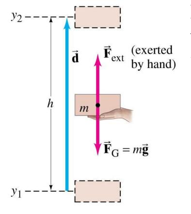
In raising a mass *m* to a height *h*, the work done by the gravitational force is
